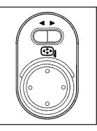
The outside power mirror controls are located on the driver's side of the vehicle next to the shift lever.
